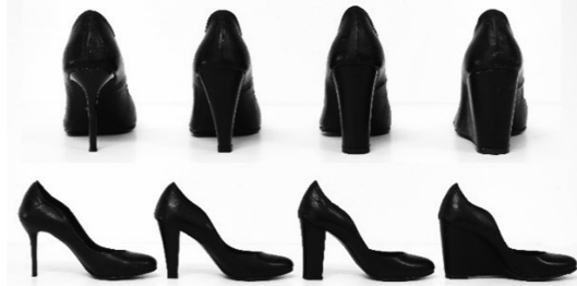
Fig. 1. The manufactured shoes (Narrow heels: 0.9 * 0.9 cm, Moderate heels: 1.5 * 1.7 cm, Wide heels: 2.8 * 2.9 cm, Wedge heels: one piece of the sole and the heel)
