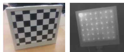
Figure 2. Heating chessboard for thermal camera calibration
