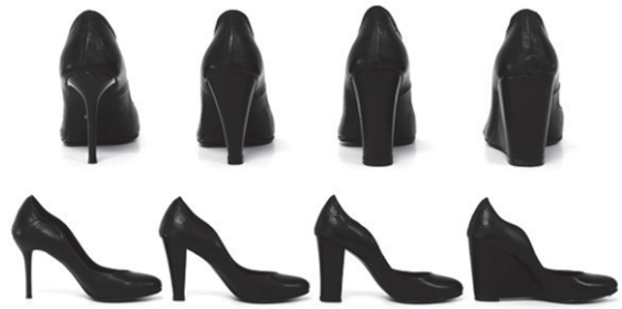
Fig. 1. Four manufactured high heels with different heel areas; from left to right, narrow heels ( 0.9 \text{ cm} \times 0.9 \text{ cm} ), moderate heels ( 1.5 \text{ cm} \times 1.7 \text{ cm} ), wide heels ( 2.8 \text{ cm} \times 2.9 \text{ cm} ), and wedge heels (one-piece of the sole and heel).
