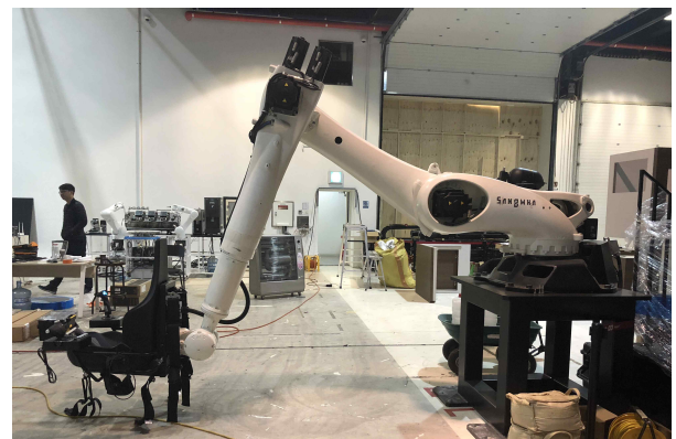
[그림 1] Experiential boarding robot equipped with an aboard in an industrial robot
